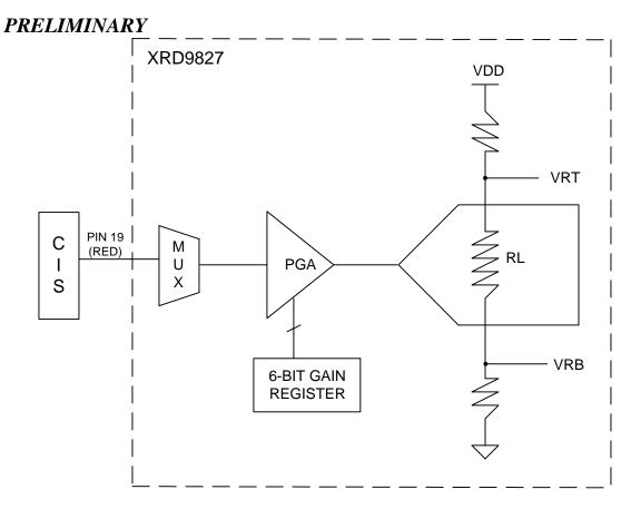
Figure 12. Simplified Block Diagram Showing Gain Adjustment by XRD9827
